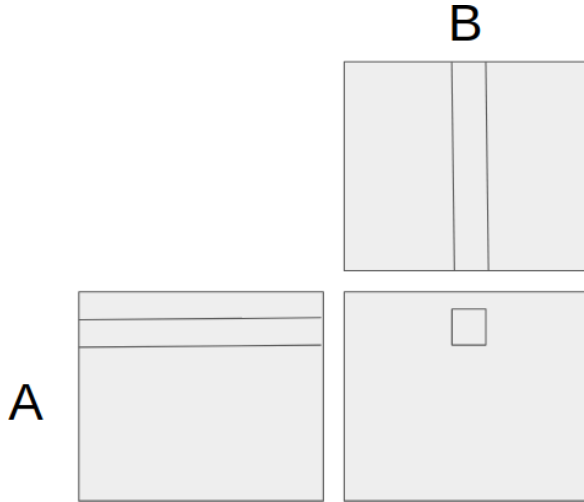
Fig. 2. The naive matrix multiply computation. Each row and column is accessed sequentially.
