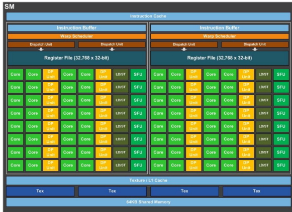
Fig. 1. The P100 SM architecture. Each SM consists of 56 cores and has its own L1 cache and shared memory. This diagram is taken from [NVIDIA 2016].
